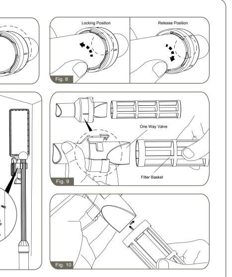
1. Twist the suction nozzle clockwise or anticlockwise to the release position, and then pull it out from the lower tube collar. (See Fig.8) 2. Grasp the plastic area at the base of the filter basket (DO NOT GRASP THE FILTER BASKET SCREEN). Rotate it anticlockwise until you feel it
