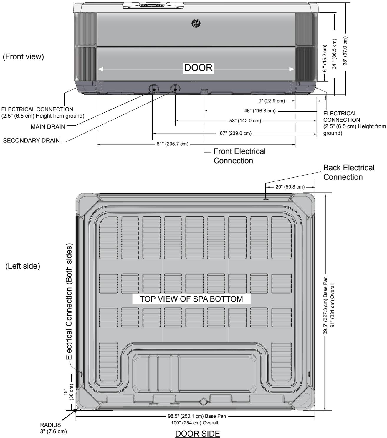
**NOTE: WATKINS WELLNESS** requires that the **GRANDEE** be installed on a minimum 10 cm (4") thick reinforced concrete pad or a deck that is able to withstand more than 555 kg/m<sup>2</sup> (125 lbs. per square foot).
