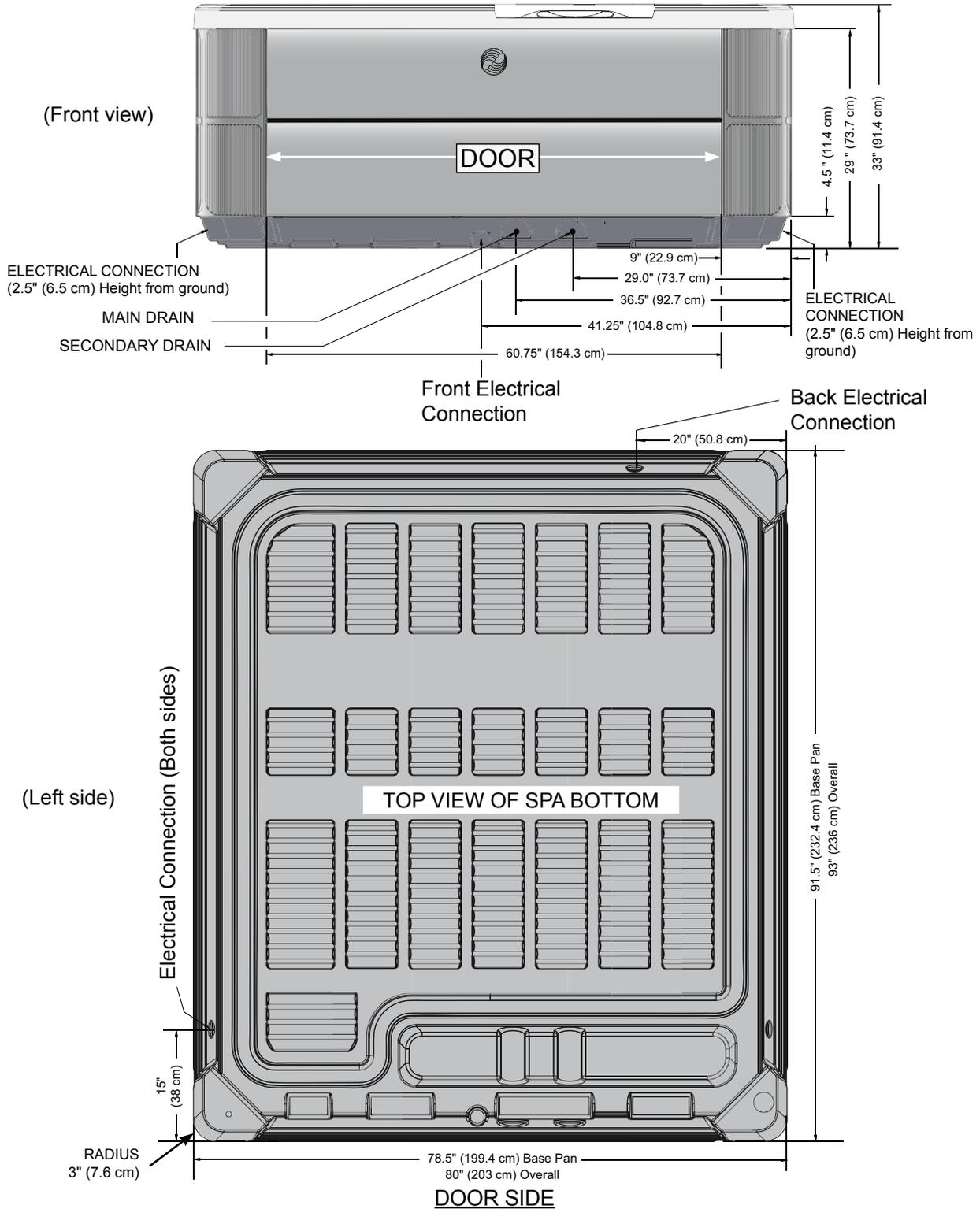
**NOTE: WATKINS WELLNESS** requires that the **SOVEREIGN** be installed on a minimum 10 cm (4") thick reinforced concrete pad or a deck that is able to withstand more than 530 kg/m<sup>2</sup> (110 lbs. per square foot).
