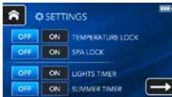
When activated, the exterior lights of the spa will come on 5 seconds later and will remain lit for 6 hours and repeat the cycle every 24 hours from activation time.
