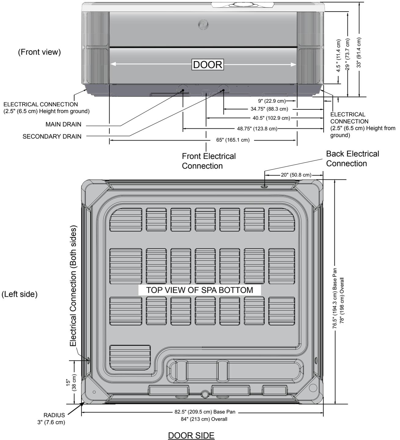
**NOTE:** WATKINS WELLNESS requires that the **PRODIGY** be installed on a minimum 10 cm (4") thick reinforced concrete pad or a deck that is able to withstand more than 595 kg/m<sup>2</sup> (125 lbs. per square foot).
