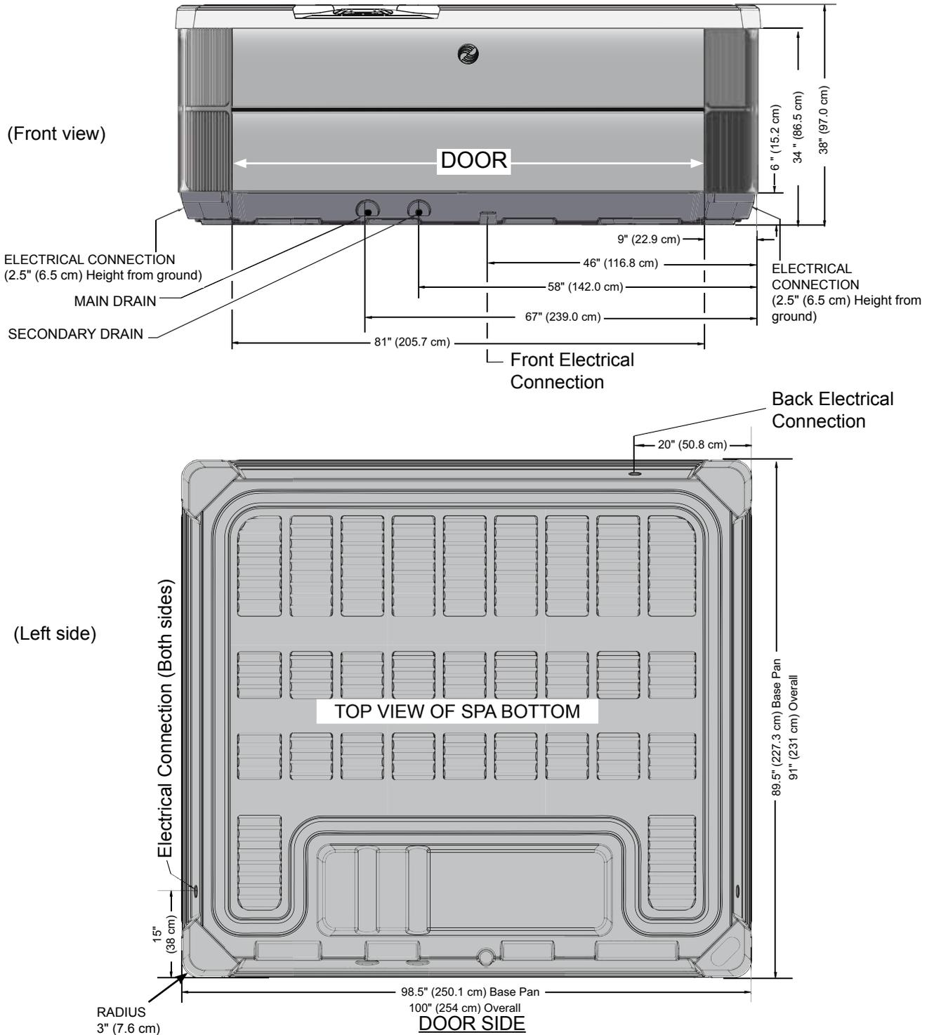
**NOTE: WATKINS WELLNESS** requires that the **ENVOY** be installed on a minimum 10 cm (4") thick reinforced concrete pad or a deck that is able to withstand more than 565 kg/m<sup>2</sup> (115 lbs. per square foot).
