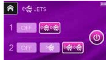
**NOTE:** If jets are off when
