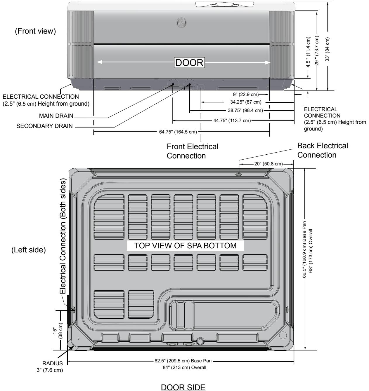
**NOTE: WATKINS WELLNESS** requires that the **JETSETTER** be installed on a minimum 10 cm (4") thick reinforced concrete pad or a deck that is able to withstand more than 460 kg/m<sup>2</sup> (95 lbs. per square foot).
