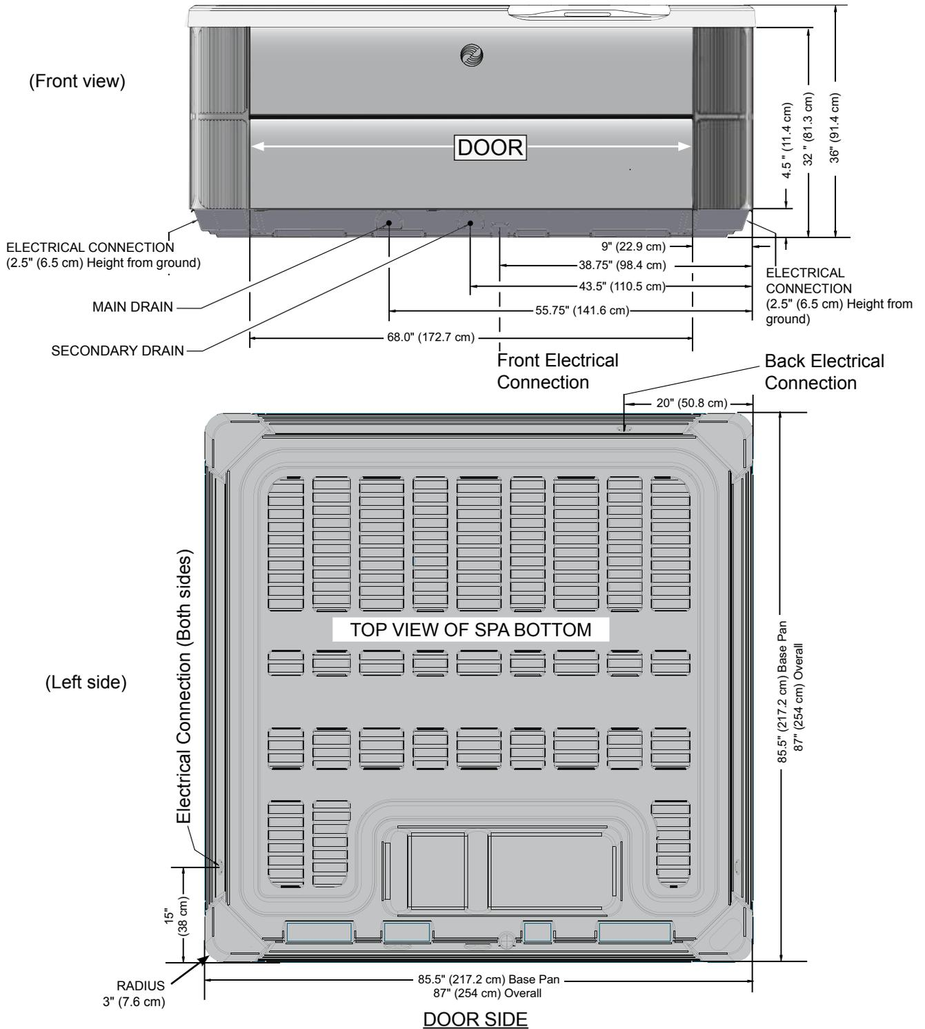
**NOTE: WATKINS WELLNESS** requires that the **VANGUARD** be installed on a minimum 10 cm (4") thick reinforced concrete pad or a deck that is able to withstand more than 565 kg/m<sup>2</sup> (115 lbs. per square foot).
