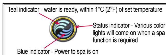
**Ready Teal Indicator:** The TEAL indicator will light when the spa water temperature is within 1°C (2°F) of the set temperature, and will turn off when the temperature is outside of that range. If you increase or decrease the temperature setting of the spa, the ready indicator will turn off until the water temperature reaches the acceptable range for the new temperature setting.
