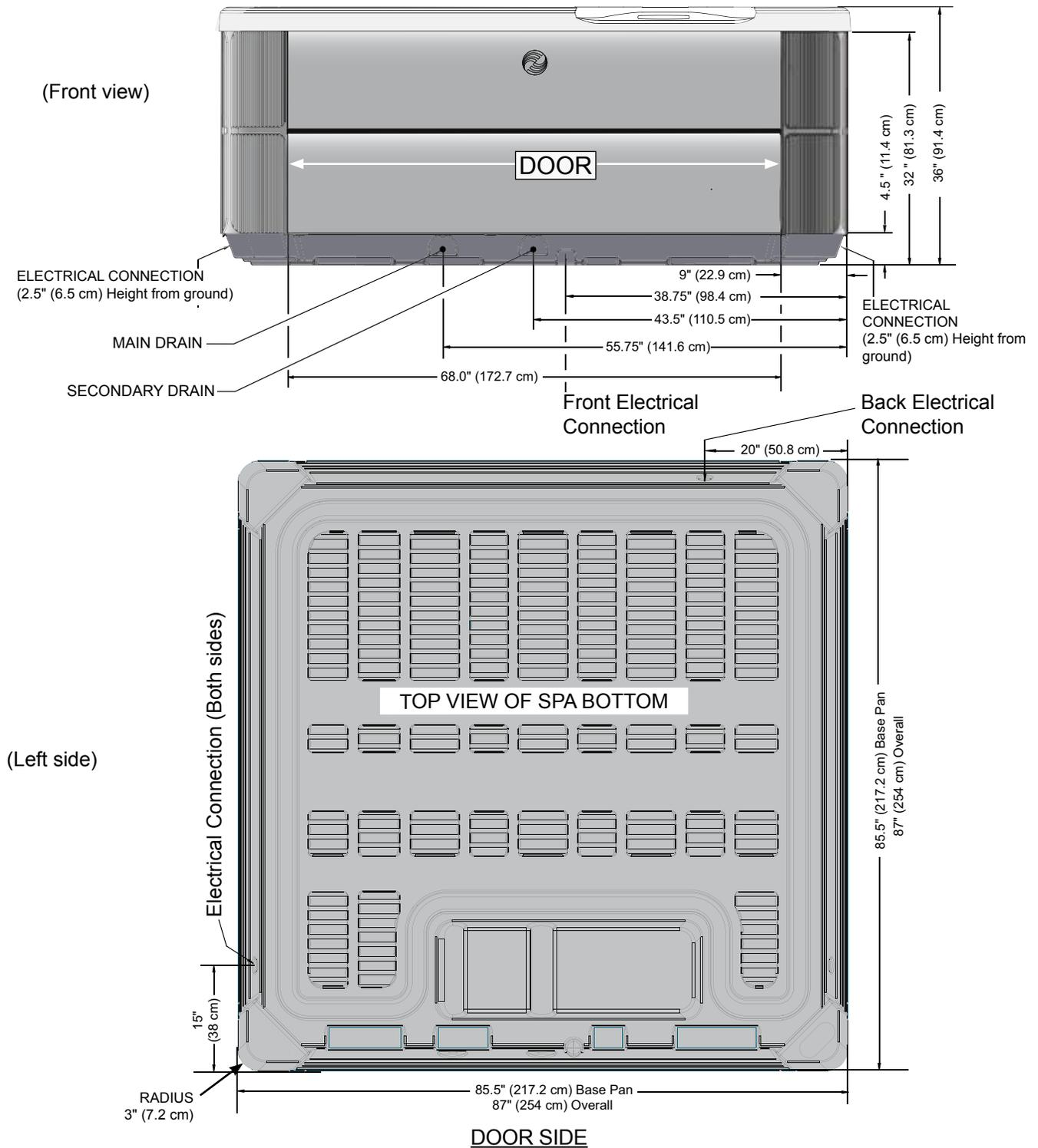
**NOTE:** WATKINS WELLNESS requires that the ARIA be installed on a minimum 10 cm (4") thick reinforced concrete pad or a deck that is able to withstand more than 565 kg/m<sup>2</sup> (115 lbs. per square foot).
